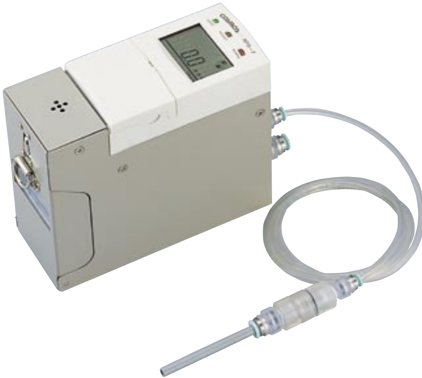
Lift the snap lock and open the sensor cover.
